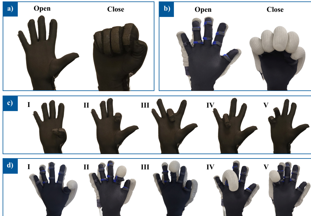
Figure 5.5 : a) Sensing T-IoT glove calibration and fist movement: open hand and close hand. b) Actuating T-IoT glove calibration and fist movement: open hand and close hand. c) Sensing T-IoT Glove single finger closing and opening: I. Thumb, II. Index, III. Middle, IV. Ring, V. Pinkie. d) Actuating T-IoT Glove single finger closing and opening: I. Thumb, II. Index, III. Middle, IV. Ring, V. Pinkie.
